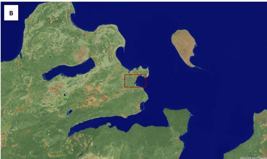
Figure 1. An example of how the spatial resolution of raster data has a direct effect on positional accuracy. LANDFIRE 30-meter resolution data does not precisely depict the shoreline or the boundary between grass (yellow shade) and forest (green shade) when viewed at a small extent (A), but at a broader extent (B), these differences are less apparent and less significant. The red rectangle in panel B shows the extent of panel A.
